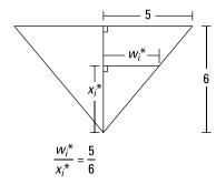
Let n be the number of subintervals of length  $\Delta x$  and let  $x_i^*$  be a sample point in the ith subinterval. Consider a horizontal slice of water that is  $\Delta x$  feet thick and is  $x_i^*$  feet from the bottom of the tank with a width of  $w_i^*$ . This slice has a volume of
