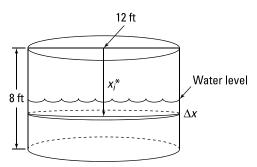
A horizontal slice of water that is  $\Delta x$  feet thick and is at a depth of  $x_i^*$  feet from the top of the tank is cylindrical, so it has a volume of  $\left(\pi(6)^2(\Delta x)\right)$  cubic feet. Because water weighs 62.5 pounds per cubic foot, this slice of water weighs 62.5(36 $\pi$ )( $\Delta x$ ) pounds. The work required to pump out this slice of water is
