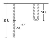
Notice that when you're lifting the end of the chain to the top, only the bottom half of the chain moves. A section of chain that is  $\Delta x$  in length and that is  $x_i^*$  feet from the middle of the chain weighs  $4\Delta x$  pounds and will move approximately  $2x_i^*$  feet. Therefore, the work required is
