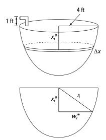
Let n be the number of subintervals of length  $\Delta x$  and let  $x_i^*$  be a sample point in the ith subinterval. Consider a horizontal slice of water that is  $\Delta x$  feet thick and is at a distance of  $x_i^*$  feet from the top of the tank; let  $w_i^*$  be the radius of the slice of water. Because the tank has a shape of a hemisphere of radius 4, you have the following relationship:
